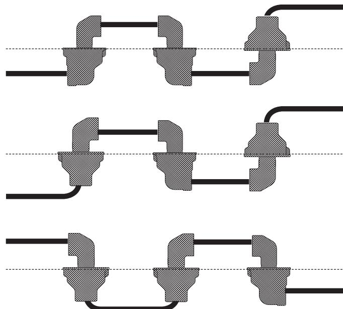
a) Knuckle Joint should be in alignment to the center line.
